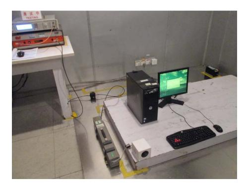
Figure B-6 EUT Setup for Conducted Immunity of DC output port
