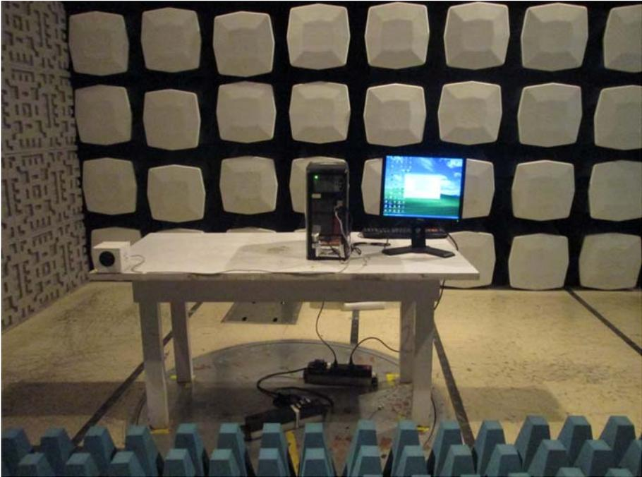
Figure B-4 EUT Setup for Radiated immunity
