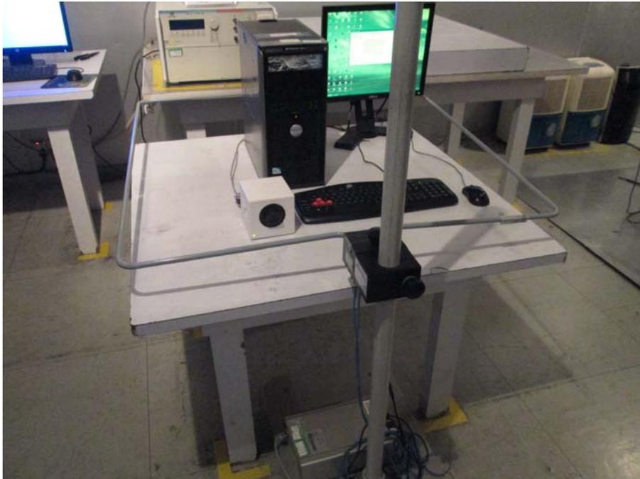
Figure B-7 EUT Setup for 50/60 Hz Magnetic Field
