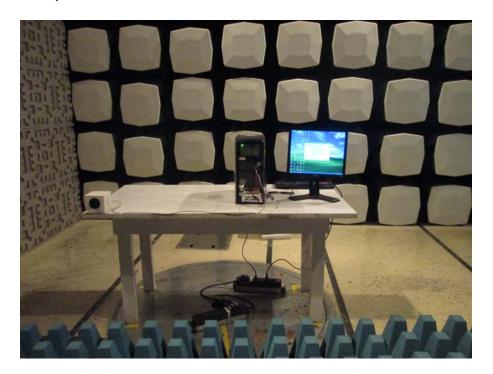
Figure B-4 EUT Setup for Radiated immunity
