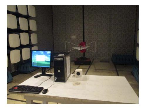
Figure B-2 Setup for Radiated emission
