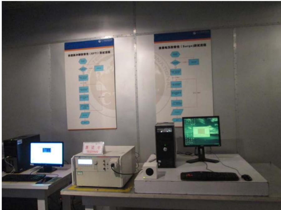
Figure B-5 EUT Setup for EFT of AC Input port
