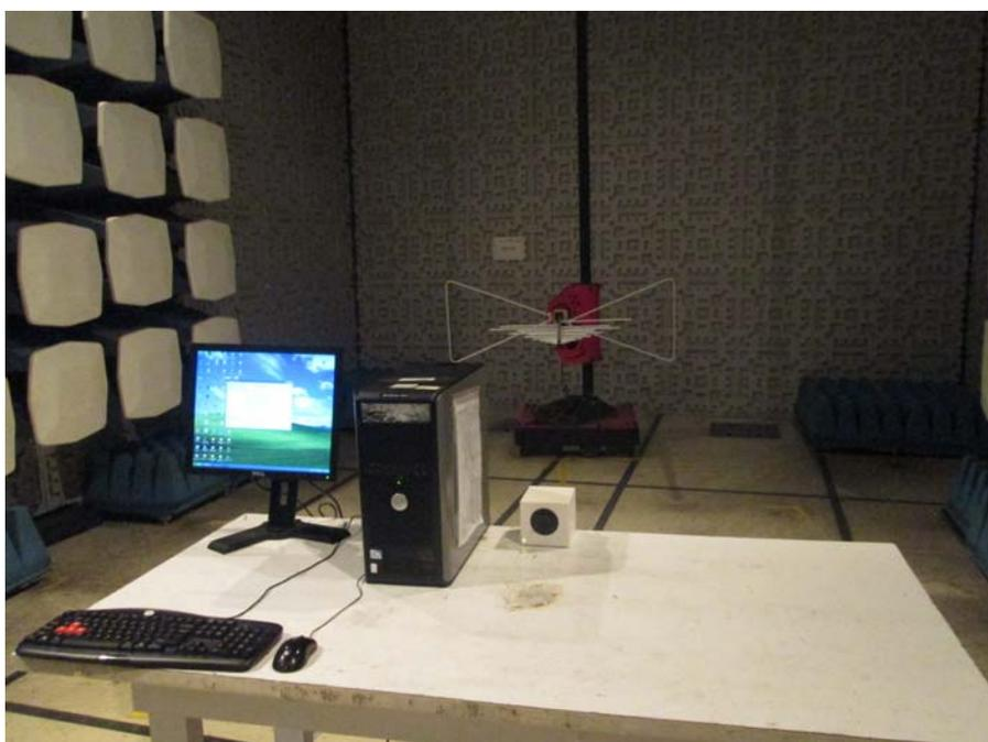
Figure B-2 Setup for Radiated emission
