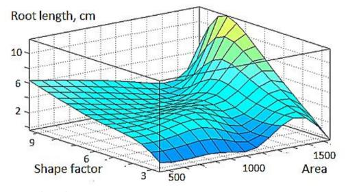
Fig. 4. ANFIS surface after training that describes the relationship between glow area, shape factor, and root length.
