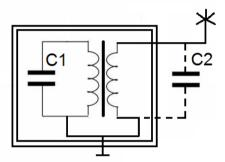
Fig. 2 Equivalent circuit diagram of the experimental setup, where C1 corresponds to the capacity of the electronic circuit of the GDV device, C2 - the equivalent capacitance of the antenna in the premises.
