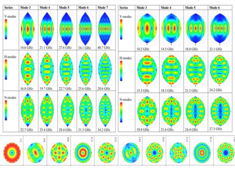
Figure 4 Resonant modes in elliptical and spherical resonators generated by finite element analysis and the resonant frequencies in GHz; V, vertical, H, horizontal, N, nodal (rearranged from [20])
