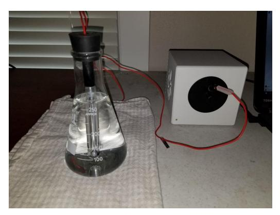
Figure 3: ORP Sensor in Flask connected to Bio-Well
