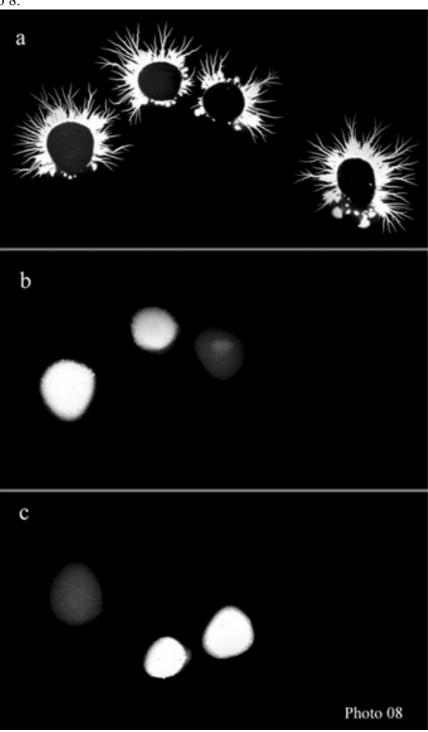
In the upper part of photo (photo 8a) there is photograph of surface discharge, which is made by traditional method of kirlian-photography. In the middle part and in the low part (photos 8b,c) – photographs of light, which are developed on the second remote film (distant plasmagraphy). In our experiments we use bilateral roentgen film, and so here is indications for remote film: b – for upper side and c – for low side.
