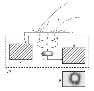
**Fig. 2.** Scheme of the GDV device. (1) Object of examination; (2) transparent electrode; (3) gas discharge; (4) optical emission; (5) generator; (6) optical system; (7, 8) video transformer; (9) computer; (10) case.
